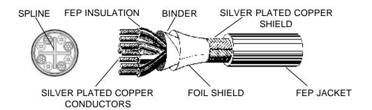
This cable has been specially designed by PIC for airborne 10- and 100Base-T Local Area Network applications as defined by ARINC Specification 646. The twisted-pair construction (four separate pairs) effectively reduces inductive interference while 100% foil and 92% braided shielding serve to further protect against EMI.
